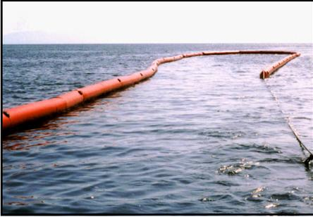
High buoyancy ensures AirBoom is suitable for use in a wide range of conditions, including open water
