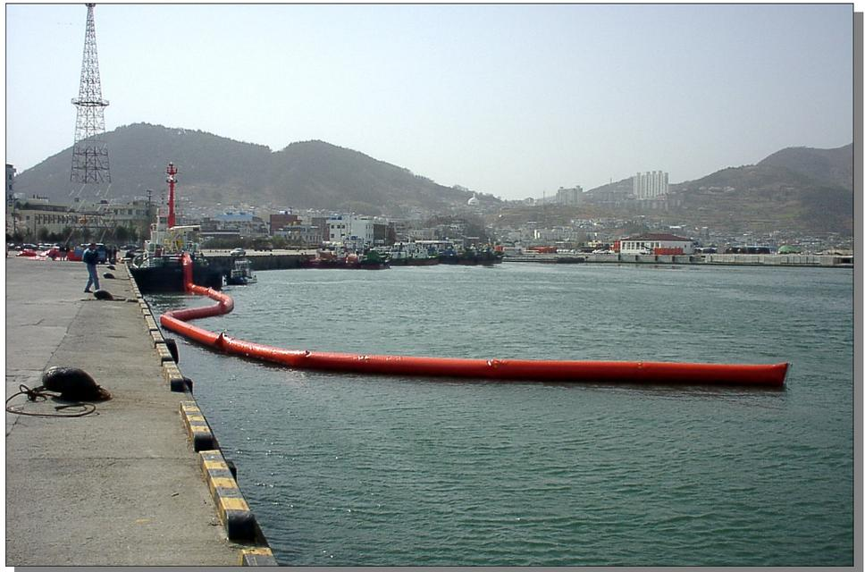
Canadyne **AirBoom SCS** is a unique inflatable boom which combines the benefits of a pressure inflatable boom with the safety and reliability of a foam filled boom. The design ensures the boom maintains positive buoyancy at all times. The boom cannot sink, and can be fully deployed and offer effective initial containment even prior to inflation. Storage on boom reels allows for easy deployment, retrieval and transportation.
